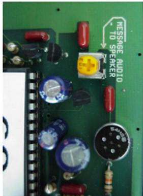
The message audio level has been pre-programmed. If the call box is located in a high-noise environment, an adjustment may be required. While holding the “RECORD-PLAY” switch (right toggle) in the down position, adjust the “MESSAGE AUDIO TO SPEAKER” control to obtain the desired level for the faceplate speaker.
