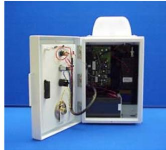
Check that the microphone and wiring harness are still connected to the circuit board as shown below.
